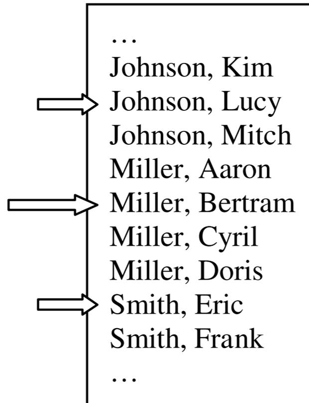
Fig. 3.6 Finding a separator key during a leaf split.
