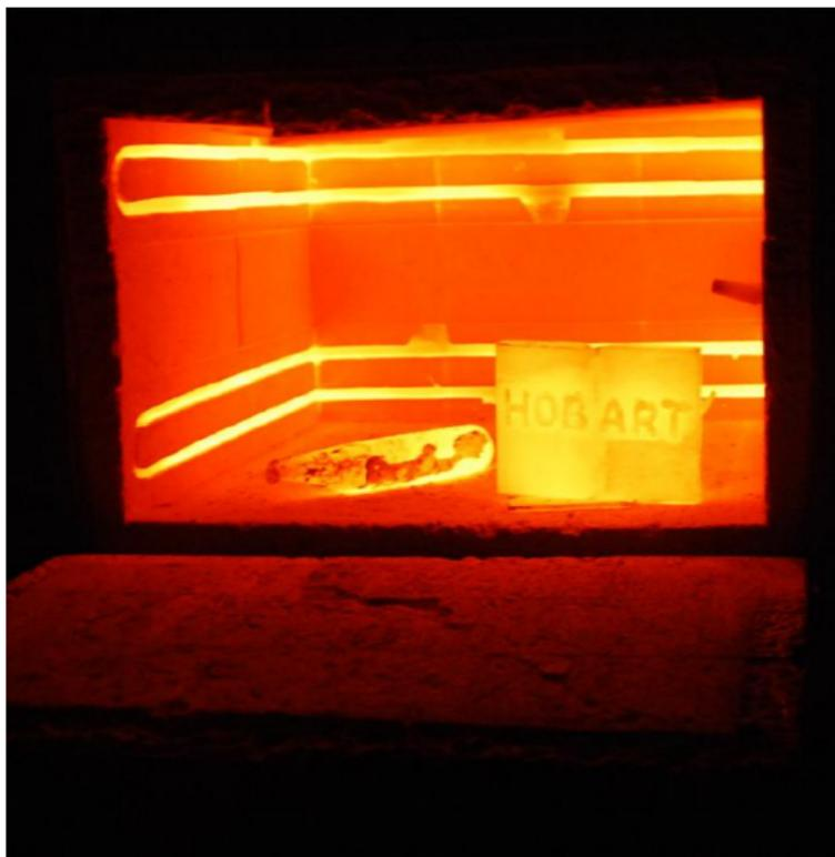
Annealing (...) is a process that produces conditions by heating to above the re-crystallisation temperature and maintaining a suitable temperature, and then cooling.
